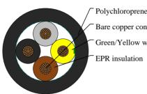
Polychloroprene rubber outer jacket Bare copper conductor Green/Yellow wire EPR insulation
